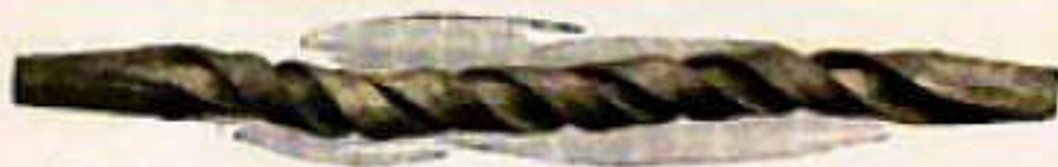
The Vanadium steel Front Axle of the Ford Car may be twisted, turned, or even bent double without showing the slightest break or fracture of the steel
