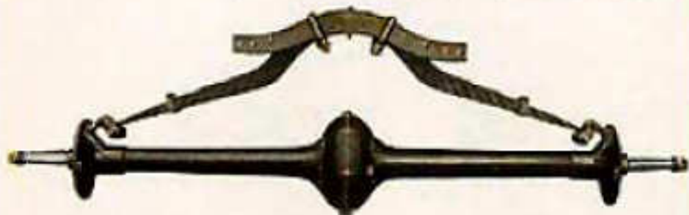
Ford Rear Axle completely enclosed in dust proof and oil proof housing
