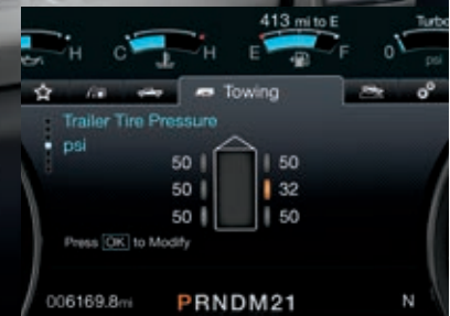
Trailer Tire Pressure Monitoring Screen
