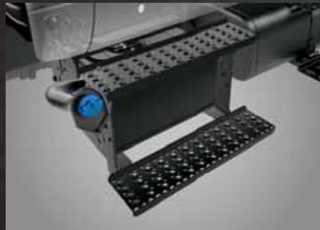
CREW CAB 10-GAL. DEF TANK option mounts under the cab on the passenger side.
