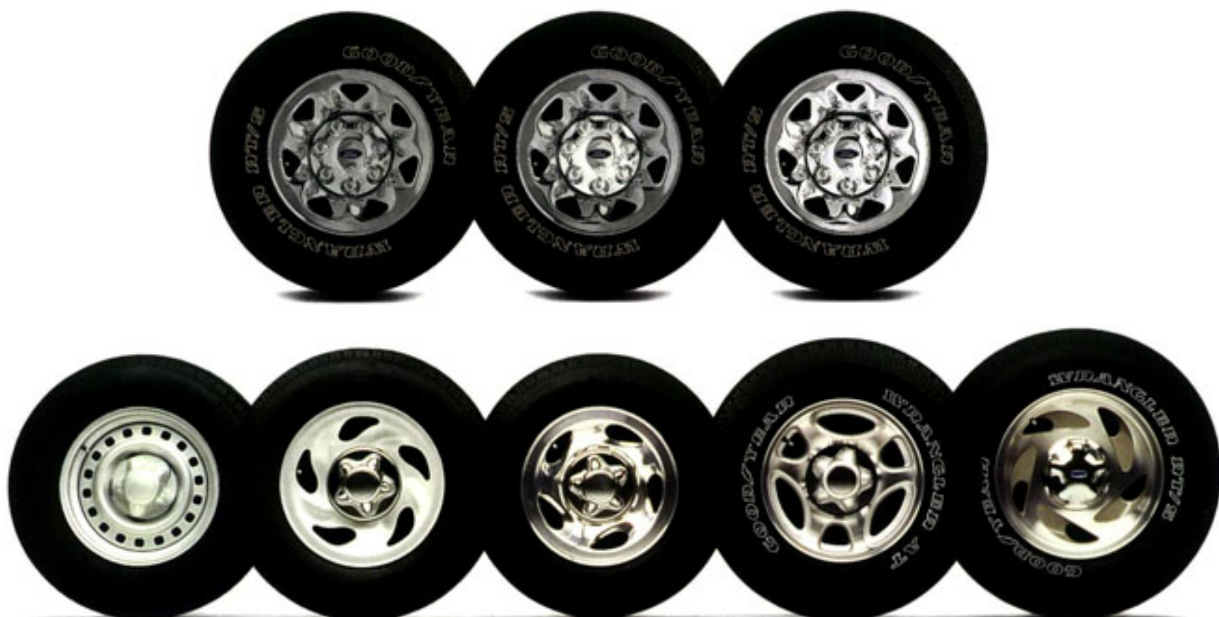
Top row wheels (OWL tires), left to right (F-250): 16" argent styled steel with argent hub, 16" argent styled steel with chrome hub, 16" chrome steel with chrome hub. Bottom row wheels, left to right (F-150): 16" argent painted steel with argent hub, 16" argent styled steel with chrome hub, 16" polished aluminum with chrome hub (BSW tires); 16" cast aluminum with chrome/argent hub (OWL tires); and 17" cast aluminum with chrome hub (included in the optional 4x4 Off-Road Equipment Group).
