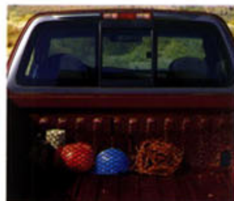
This cargo net secures items like tools and hard hats inside the pickup box.
