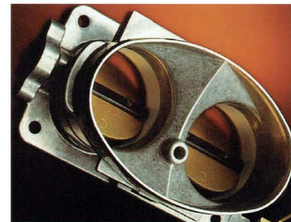
Unique to Cobra is a throttle body with twin 57mm bores. The bores open simultaneously, not in stages, giving the engine exceptional throttle response by quickly yet progressively delivering large volumes of air to the cast alloy plenum that sits atop the Cobra engine.
