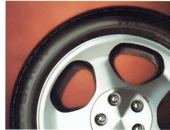
The Cobra's 17.0-inch five-spoke alloy wheels are wrapped with BFGoodrich Comp T/A ZR radials, which are derived from the Comp T/As fitted to SVT's 1995 Mustang Cobra R race car.
