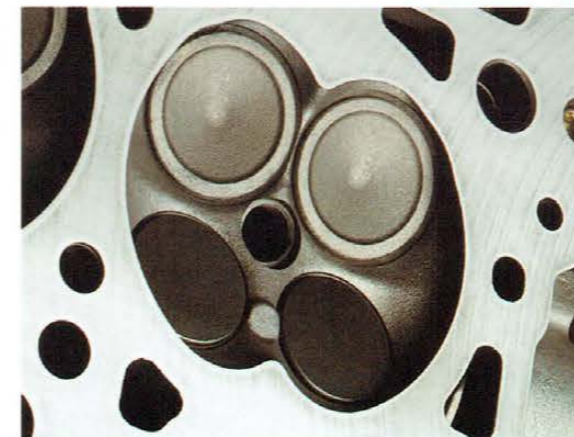
The curved lip around the inlet for the primary intake valve directs the fuel-air mixture as it enters the combustion chamber, causing it to swirl.
