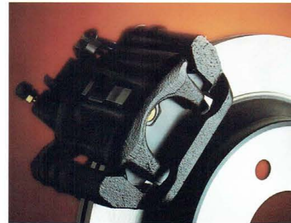
The 11.65-inch rear brakes are clamped by single-piston calipers. The rotors feature internal cooling vanes.
