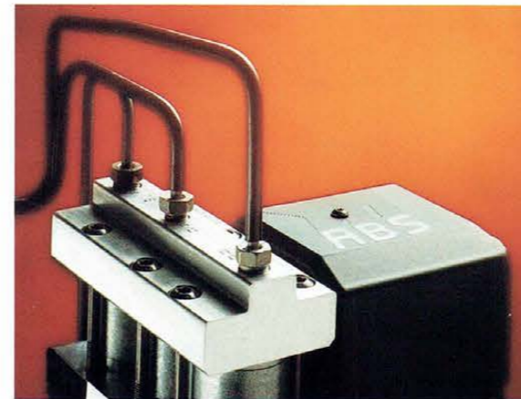
The Cobra's brakes are monitored and controlled by a three-channel, four-sensor Bosch ABS system that can modulate and adjust each of the four calipers every 10 milliseconds.
