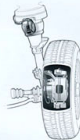
Continental's computer-managed suspension system can change from a soft to firm damping rate in milliseconds based on inputs from sensors in the brakes, suspension and engine.
