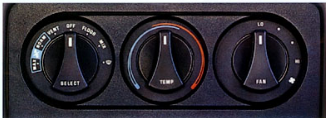
Air conditioning with rotary controls.
