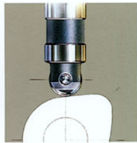
Roller tappets in the 5.0L help reduce friction and heat.
