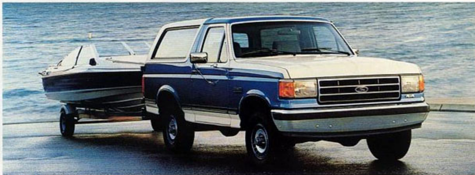
Bronco XLT with optional Trailer Towing Package, 5.0L engine and 4.10 rear axle ratio (automatic overdrive transmission) has a towing capacity of 7,800 pounds.
