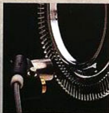
Mark's Anti-lock Brake System begins with a speed sensor at each wheel that sends information to a microprocessor.
