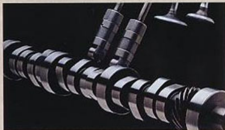
One example of applied racing technology is low friction roller tappets.
