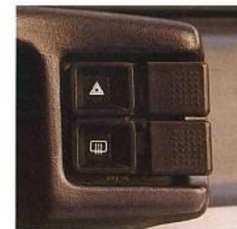
Control pods for running lights, flashers and rear defroster are placed within clear view and easy reach.
