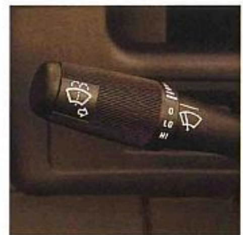
The interval wiper/washer, high beam and flash-to-pass control is at your fingertips.
