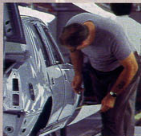
An inspector goes over a randomly selected vehicle inch-by-inch to check on fit and finish.
