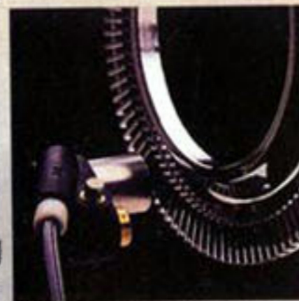
Mark's Anti-Lock Brake System begins with a speed sensor at each wheel that sends information to a microprocessor.
