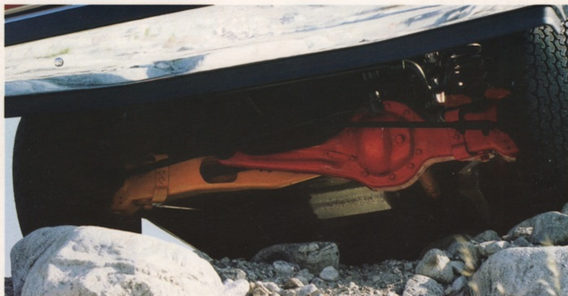
Above: Twin-Traction Beam independent front suspension. (Some items painted for display purposes.)
