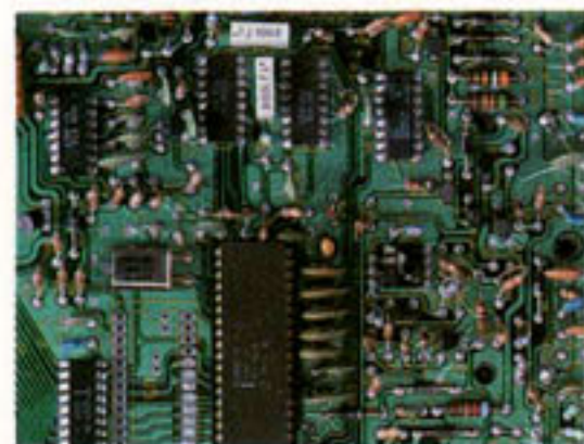
Engine functions are monitored and controlled by the advanced EEC-IV computer.
