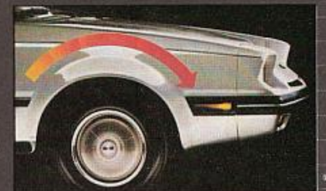
Front-wheel drive puts the weight over the driving wheels for traction.
